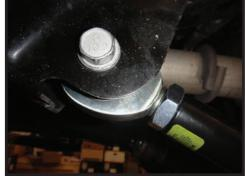
5. Once installed, torque jam nut to 300 ft-lbs.
